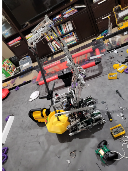
Workshop mobile-goal lift test; the clamp at left was installed on this robot.
